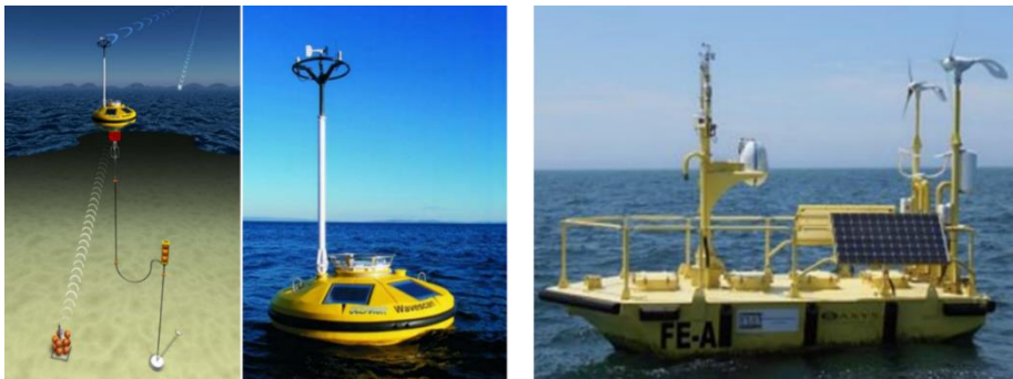
Photo 8.3 Floating Lidar buoy for measuring wind profile, etc.
