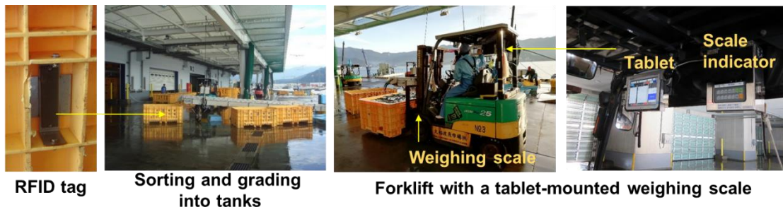
Figure 3.9 Forklift with tablet-mounted weighing scale and fish tanks with IC tags, Ofunato, Japan
